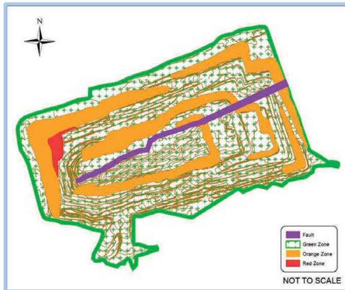
Figure 36: Geotechnical Hazard Plan (Source: Tshipi Borwa Mine)
