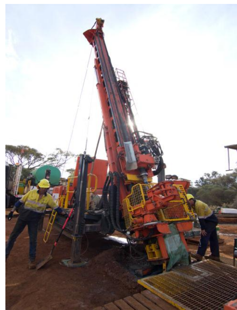
Mount Mason – Diamond drill rig
