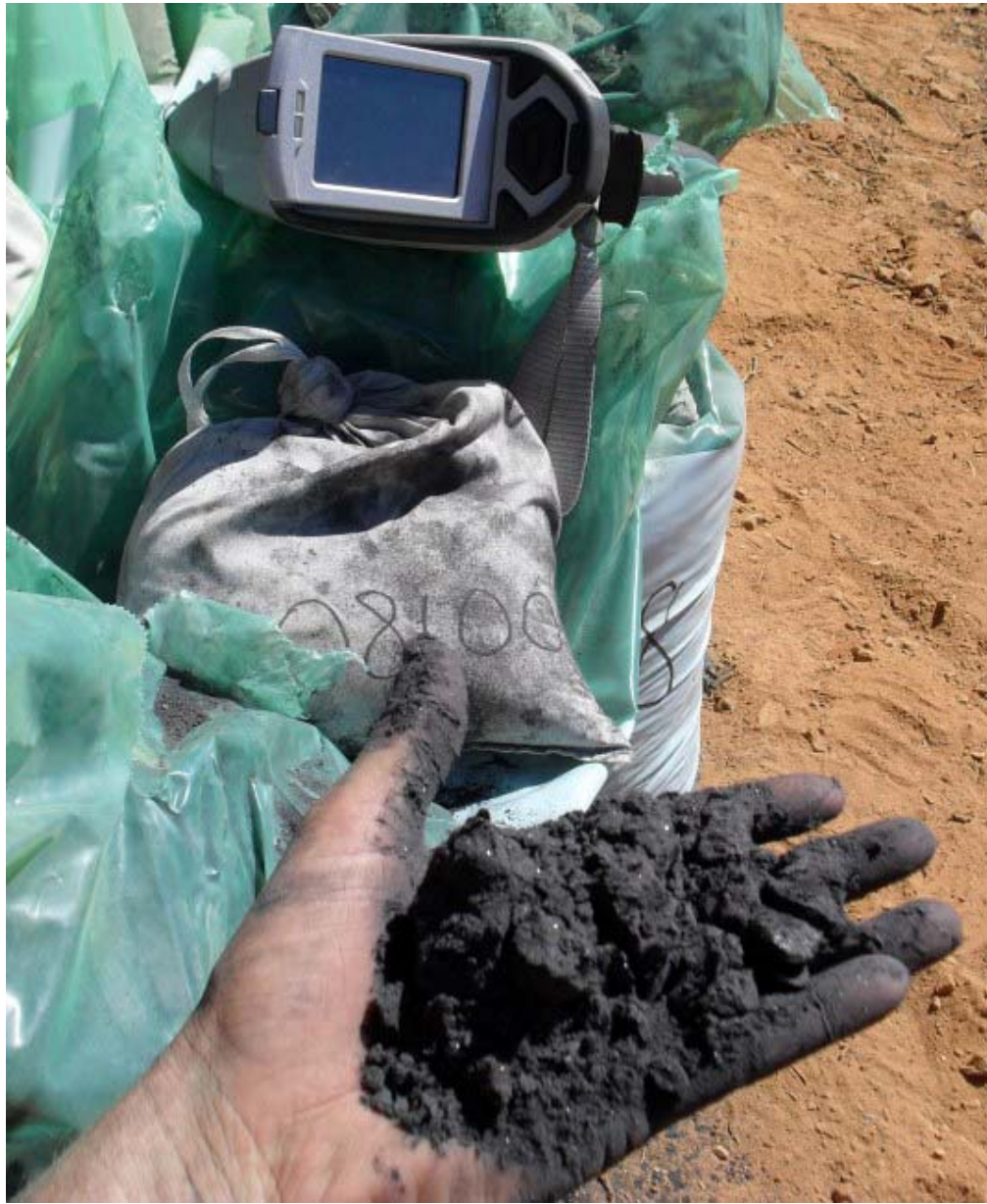
Figure 2 Coarse Magnetite RC drill cuttings from Mt Ida
