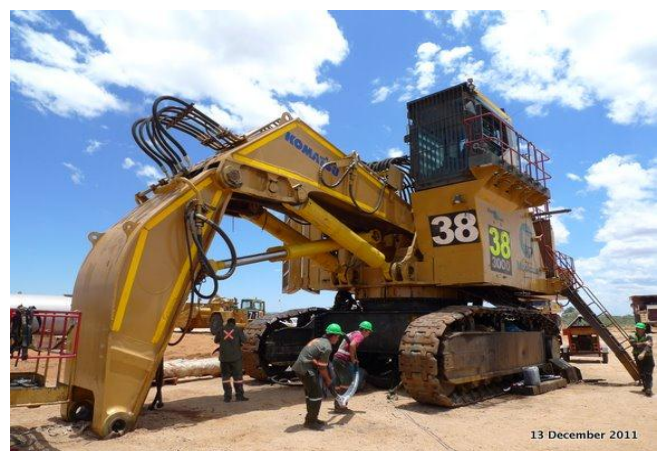
Tshipi Borwa – final assembly of excavators being completed
