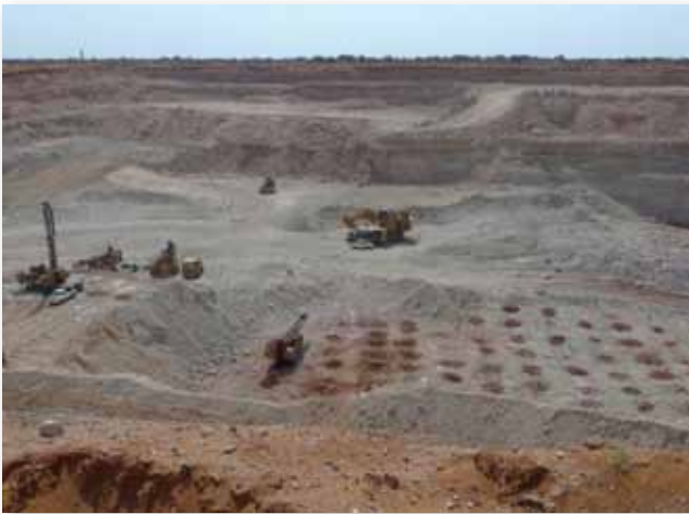
Figure 4. Tshipi Borwa – Blast Hole Drilling in Progress
